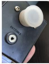
capability. These are distinguished by a screw-in antenna terminal for the FSM antenna (left).
