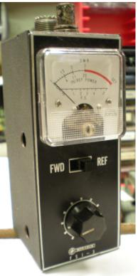
If you happen to have a vintage SWR bridge without the FSR option it is a trivial matter to add it. Simply add a connector for the FS antenna and two diodes as shown in the figure below.
