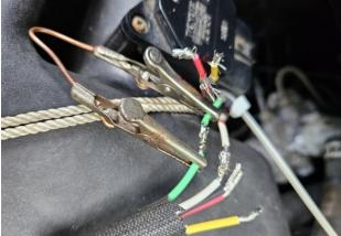
The figure at left shows my Gator Gadget holding wires for soldering. The multiple strands are spread, interleaved, and pressed together. Releasing one of the two alligator clips allows fine adjustment of the wire overlap. The Gator Gadget holds the wires together firmly while soldering, allowing a good electrical and mechanical splice (right).
