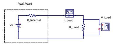
One of the wall warts in my cache is from a Korg audio gadget, and is labeled as 9V and 600mA (see picture below.) Using the test circuit described above, the wall wart was loaded with various  $R_{Load}$  values, drawing currents ranging from 0 to 600mA. The V vs I measurements are shown in the plot below.
